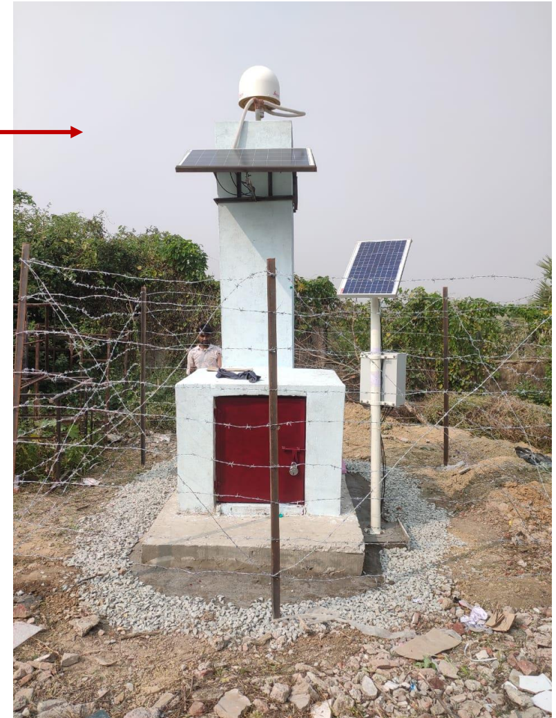
Ex. GNSS and Soil Moisture Probes Installed at INV, Aurangabad, Bihar
