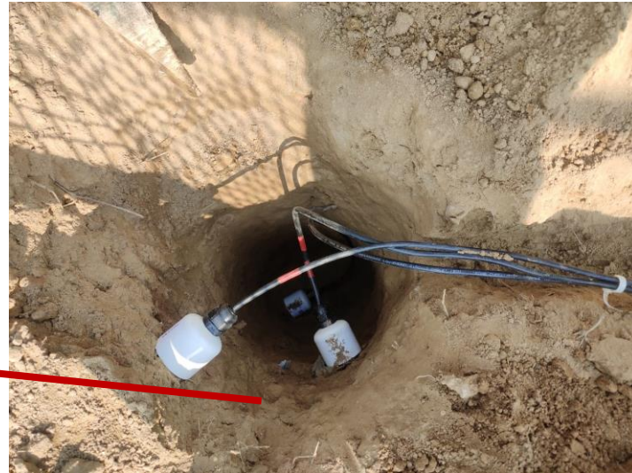
Three Hydra Probe soil sensors installed 3 distinct soil horizons.
