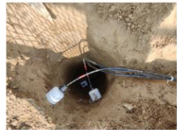
Three Hydra Probe soil sensors installed in 3 distinct soil horizons.
